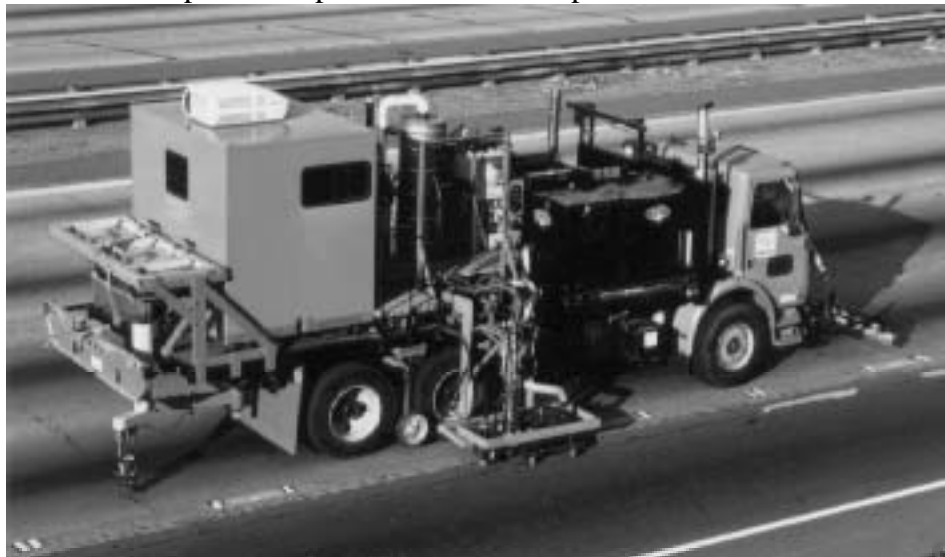
Figure 3. Automated Crack Sealing Machine developed by UC Davis.
