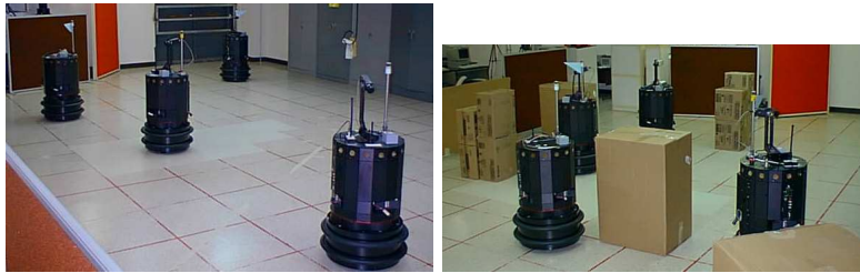
Figure 2: Robot team executing human-generated solution to CMOMMT. The first photo shows robots operating in an area with no obstacles. The second photo shows the robots amidst randomly distributed obstacles.
