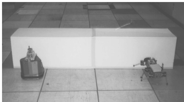
Figure 22: Adaptivity due to heterogeneity. In the second experiment, we again seize one of the R-2 robots, but this time we replace it with GENGHIS . Since GENGHIS cannot push as powerfully as an R-2, the remaining R-2 robot adapts its actions by pushing less frequently.
