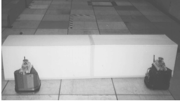
Figure 19: The beginning of the box pushing application. Two R-2s are pushing the box across the room. (The R-2 robot GREEN is on the left, the R-2 robot BLUE is on the right.)
