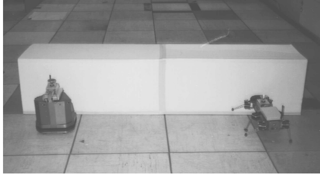
Fig. 6. Adaptivity due to heterogeneity. In the second experiment, we again seize one of the R-2 robots, but this time we replace it with Genghis-II. Since Genghis-II cannot push as powerfully as an R-2, the remaining R-2 robot adapts its actions by pushing less frequently.
