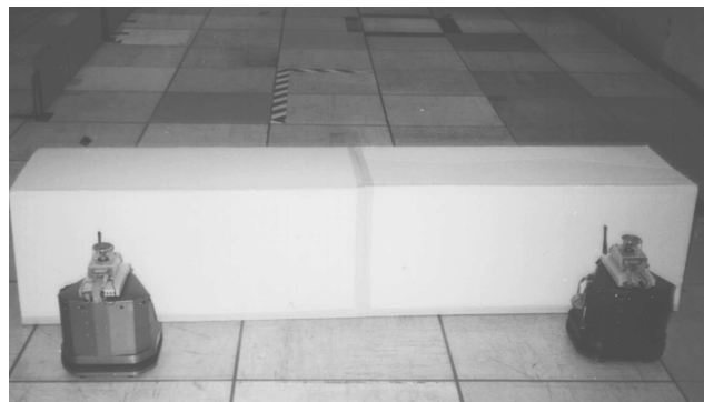
Fig. 4. The beginning of the box pushing mission. Two R-2s are pushing the box across the room.
