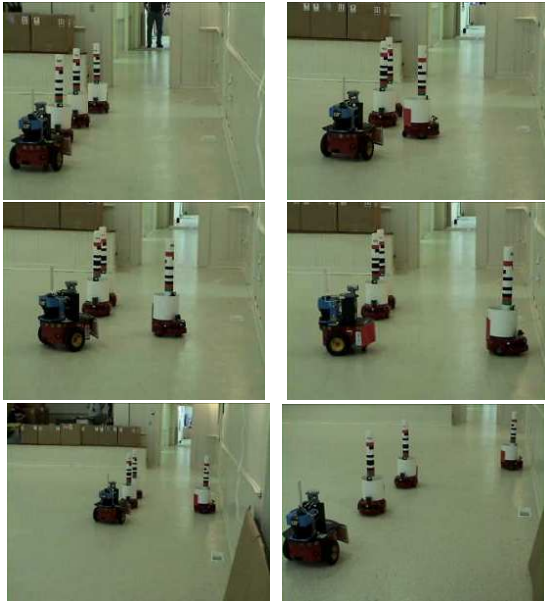
Fig. 2. [Deployment] Deployment of a sensor robot using assistive navigation: the lead robot first guides and then directs the sensor robot into position (read left to right, top to bottom).
