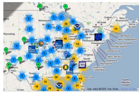
Fig. 2. The Sensorpedia Web Application’s Google map mashup illustrating Sensorpedia’s ability to cluster sensors according to a user’s current level of magnification. [2]
