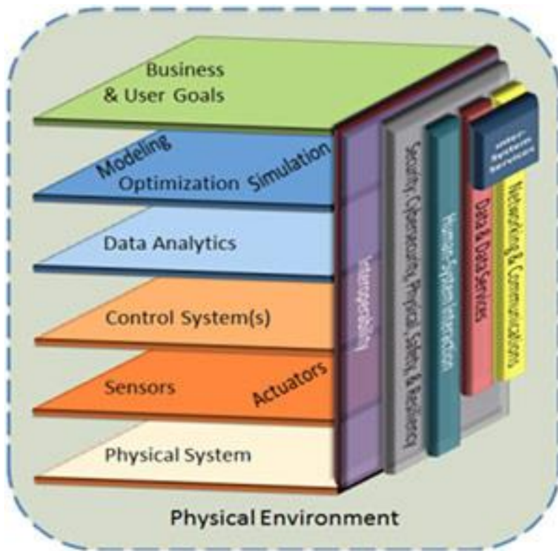
Figure 2. CPS Reference Architecture for Smart City Infrastructure
