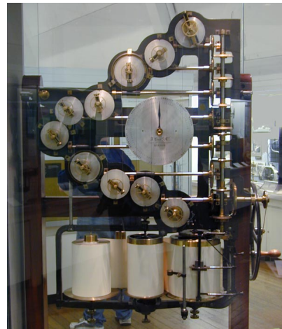
Figure V.8: Lord Kelvin’s analog tide computer. [source: wikipedia]
