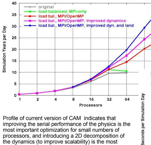
CAM performance measurements on IBM p690 cluster (and other platforms) were used to direct development process. Graph shows performance improvement from performance tuning and recent code modifications
