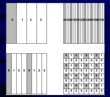
1D block-cyclic column and 2D block-cyclic distribution used in ScaLAPACK
