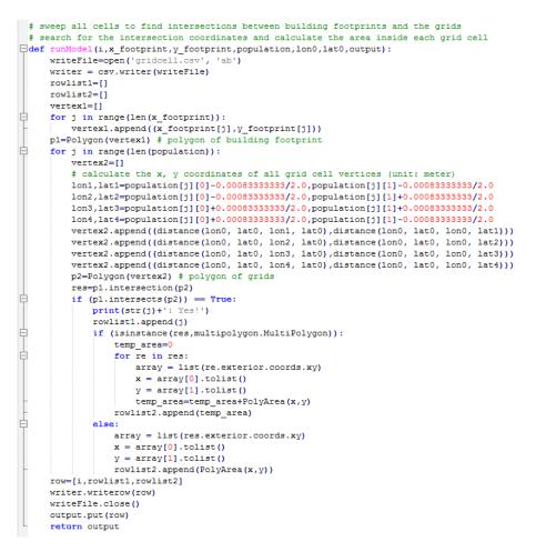
Figure 11 Code of finding intersected grid cells and area
