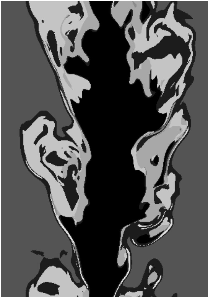
Fig. 6. SFAM network output node clustering of jet combustion data.
