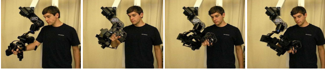
Fig. 8. Sarcos Master arm used to record a human trajectory in end-effector space. Here, the subject demonstrates a pouring movement which after learning the DMP enabled a robot to pour water into several cups (see Fig. 12).
