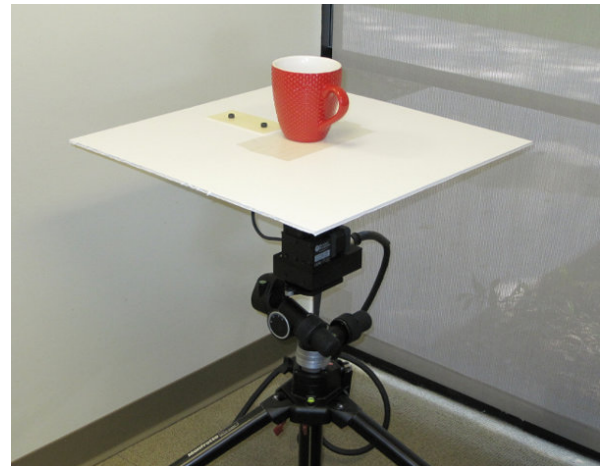
Fig. 7. The turn table used to collect views of objects with known orientation.
