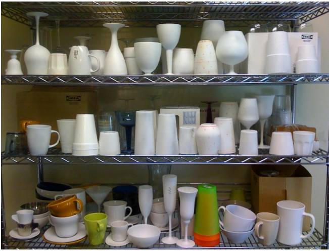
Fig. 8. The complete set of IKEA objects used for the purpose of our experiments. All transparent glasses have been painted white to obtain 3D information during the acquisition process.
