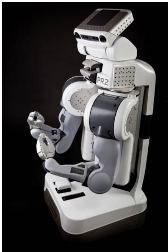
Fig. 1. A PR2 robot from Willow Garage, showing its grippers and stereo cameras
