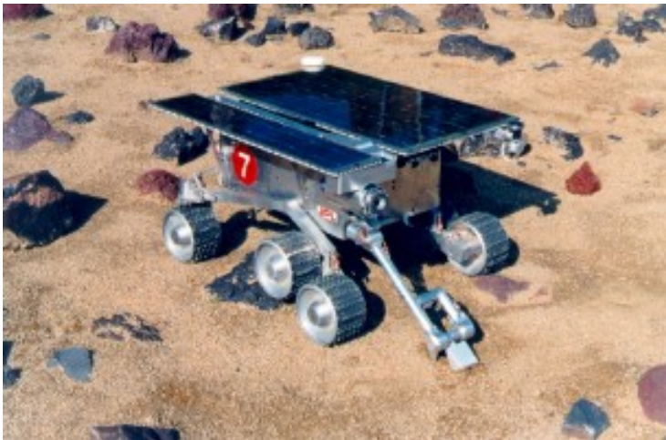
Rocky 7, with stereo vision and sampling manipulator
