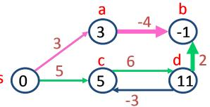
Edge weight & Path weight : Edge weight: eg. w(c,d) = 6 Path weight: eg. For a path p=<s,c,d>, w(p) = w(s,c) + w(c,d) = 11
