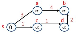
Where v.d is the upper bound on the weight of a shortest path from source vertex s to v.
