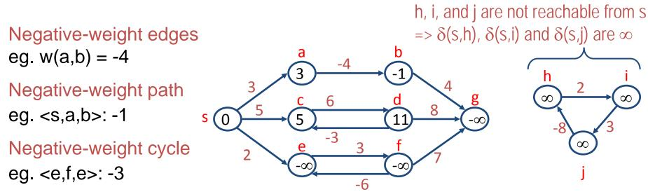
If there is no negative weight cycle reachable from the source vertex s, then for all v in V, the shortest-path weight  $\delta(s,v)$  remains well defined.
