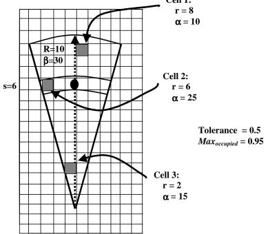
For the situation in the above diagram, supply the unconditional probability values for Cells 1, 2, and 3 below. If the value is unknown according to the sonar model update rules, then enter "Unknown".
