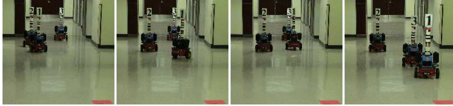
Fig. 2. Illustration of ASyMTRe dynamically forming coalitions for a cooperative navigation task. From [34].
