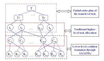
Fig. 1. The relationships between tasks, coalitions and robots.
