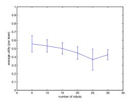
Fig. 5. The size of the robot team (n) vs. the average solution quality.
