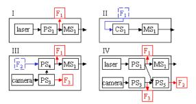
Fig. 2. Four types of robots (I, II, III, and IV) defined by various connections of schemas to accomplish the task. The dashed-line box represents the information required by the robot. The solid-line box represents the information produced by the robot. We assume that all the robots have communication capabilities and  $CS_1$  is omitted except for the type II robot.
