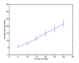
Fig. 4. The size of the robot team (n) vs. the average time to achieve solutions using parameter settings in Table III.
