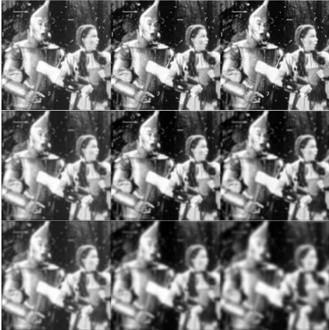
Figure 5: Spatial Gaussian Filtered Image, Frequency Gaussian Filtered Image, Frequency Butterworth Filter (order =2)(3x3, D_0 = 64; 5x5, D_0 = 32; 7x7, D_0 = 16)
