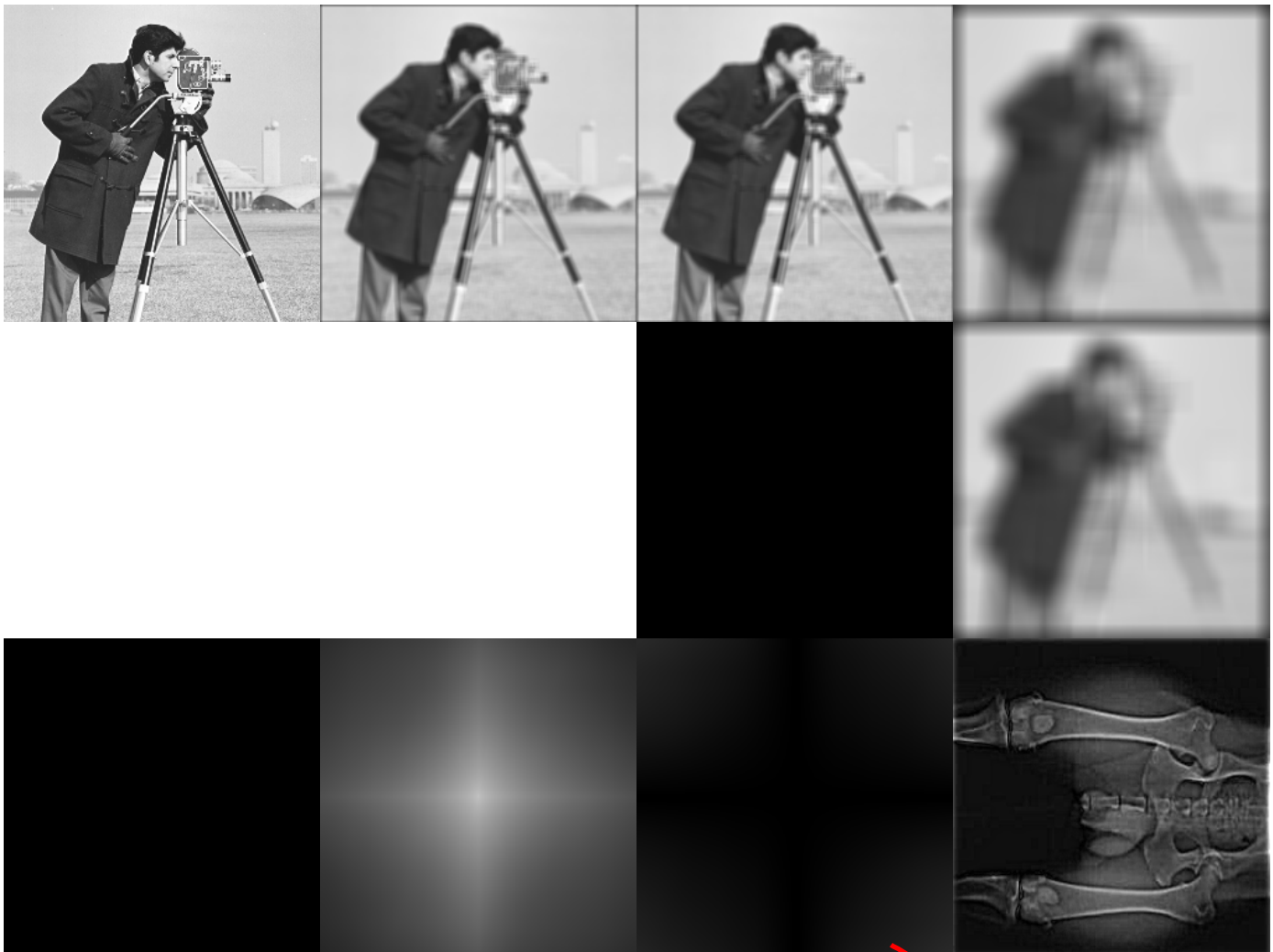
Fig. 6. The top row: original image, average filtered spatially 5x5, frequency average filtered 5x5, spatially average filtered 25x25. Second row: difference between spatial and frequency 25x25 log-scaled, difference between spatial and frequency 5x5 log-scaled, difference between spatial and frequency 5x5, frequency average filtered 25x25. Bottom row: difference between spatial and frequency for 25x25, spatial autocorrelation, frequency autocorrelation, and homomorphic filtering .
