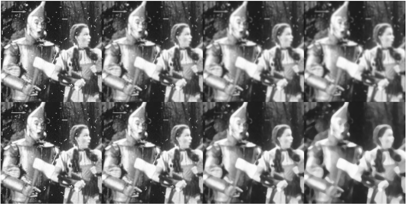
Fig. 3. The top row is Gaussian Blurring, and the bottom row is median filtering. The dimensions below correspond to the mask size used for each spatial filtering process.
