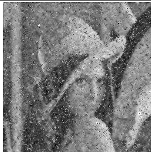
(Adaptive local noise reduction filter with variance=2550, kernel size=5) MSE: 1222.62 PSNR: 8.62894
