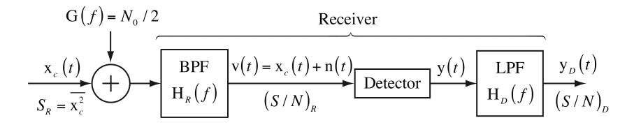
(This development is not identical to the one in the book but the final conclusions are the same.) For DSB and synchronous detection  $x_c(t) = A_c x(t) \cos(\omega_c t)$ ,
