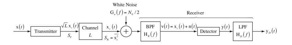
The filtered noise at the output of the bandpass filter has the power spectrum  $G_n(f) = (N_0/2) |H_R(f)|^2$ . The bandpass filter is assumed to have a nearly rectangular shape with bandwidth  $B_T$ . Therefore the
