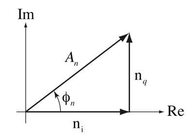
The mean value of the envelope is  $\overline{A_n} = \sqrt{\pi N_R / 2}$  and its mean-squared value is  $\overline{A_n^2} = 2N_R$ . The phase is uniformly distributed over a range of  $2\pi$  radians and is independent of the envelope.
