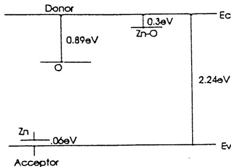
Figure 3 Energy levels in GaP: Zn-O system
