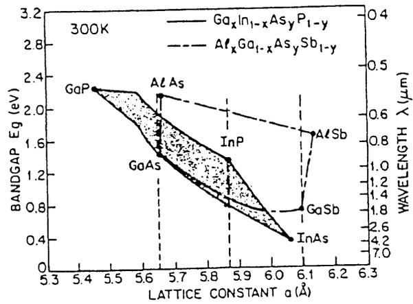
Fig. 16 Energy bandgap and lattice constant for two III-V compound solid alloy systems.<sup>1</sup>
