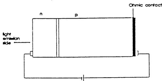
Figure 1 A forward-biased GaP diode
