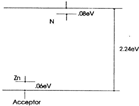
**Figure 5** Energy levels in a GaP:N,Zn system
