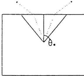
Figure 7 A schematic representation of loss due to total internal reflection.
