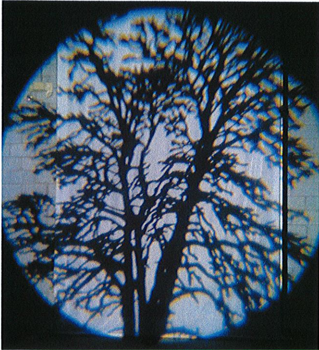
Figure 10: A tree template projected onto a wall using a halogen sourced Source 4 Ellipsoidal unit. The hard edges around the edge of the light and the template are desired for profile instruments.
