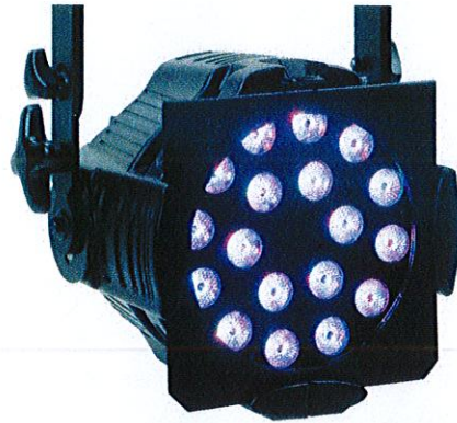
Figure 15 – The Elation Opti Tri Par with 5 W RGB LEDs. Using single chip RGB LEDs eliminates color-fringing issues.
