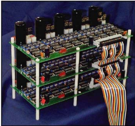
Fig. 4. Gate Driver Boards and MOSFETs for the Multilevel Inverter
