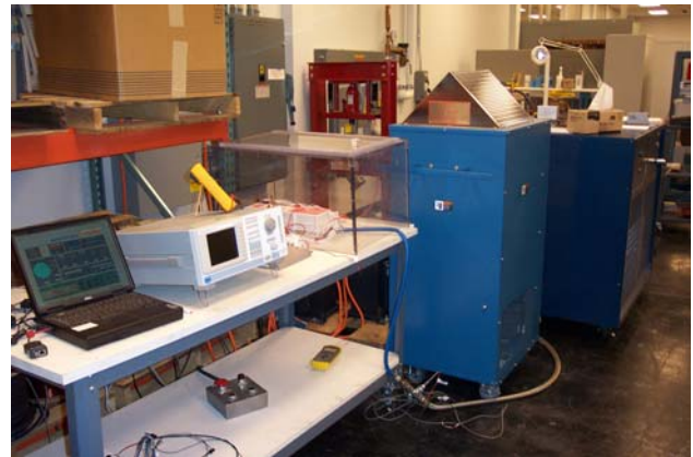
Fig. 10. Inductive load test set-up.
