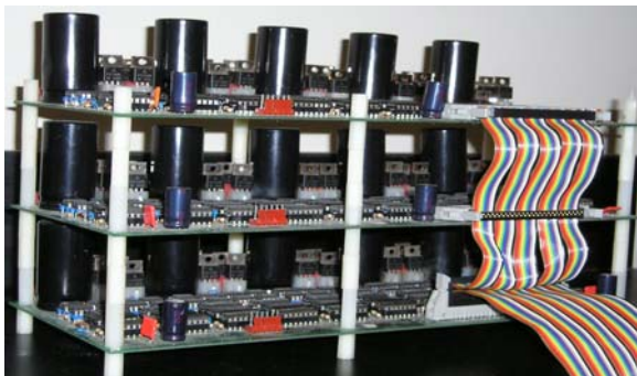
Fig. 9. 10 kW multilevel converter prototype
