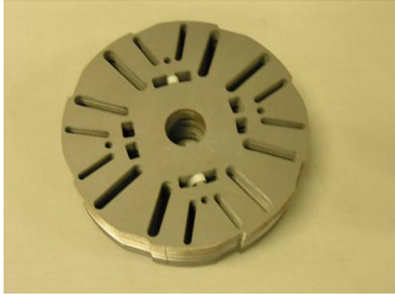
Fig. 5 Assembled rotor core stack.
