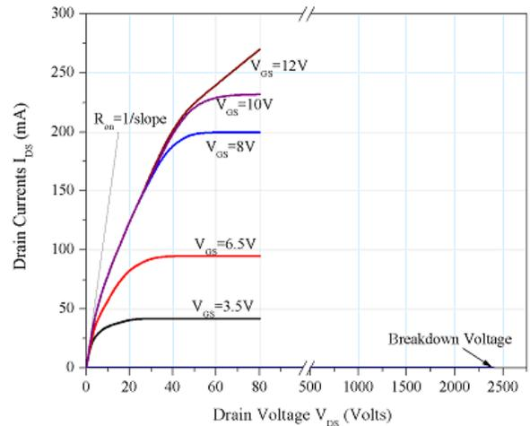
**Figure 3.** Output characteristics of the MEDICI simulations
