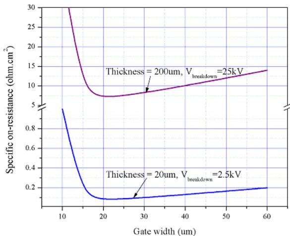
**Figure 5.** Variation of specific on-resistance with gate width
