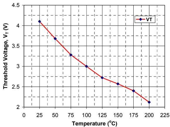
**Figure 9:** DIMOS threshold voltage,  $V_T$  variation with temperature
