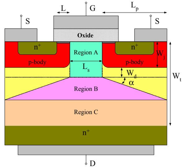
**Figure 1.** DIMOS structure for modeling. Labels describe the different regions and dimensions
