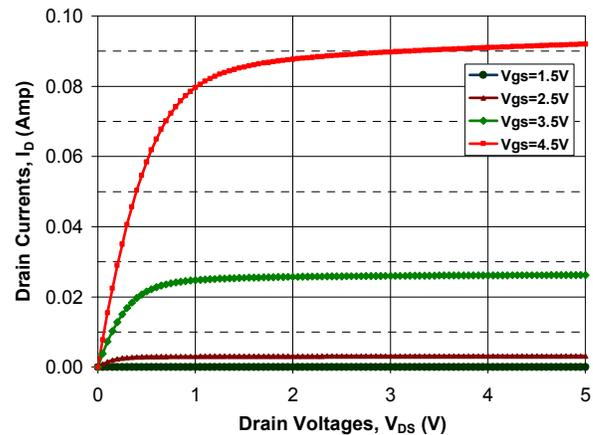
**Figure 7:** DIMOS output characteristics measured at a temperature of 200°C
