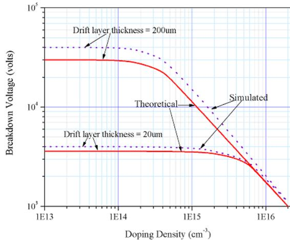
**Figure 4.** Variation of breakdown voltage with doping density
