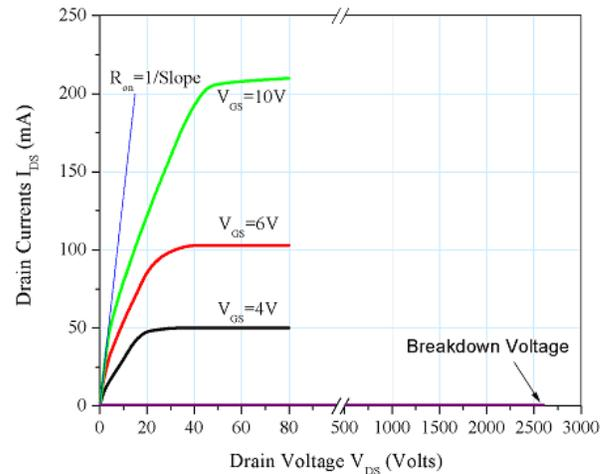
**Figure 2.** Output characteristics of the analytical model
