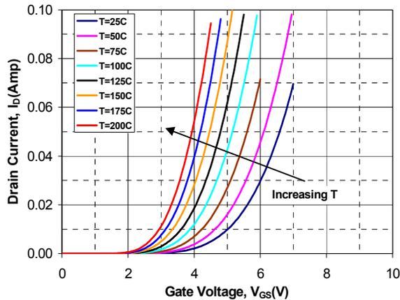
**Figure 8:** DIMOS transfer characteristics at different temperatures
