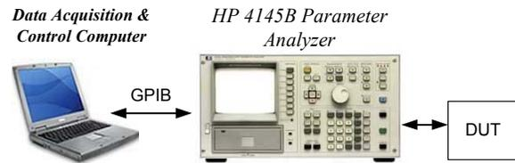
**Figure 6.** Test setup for DC characterization
