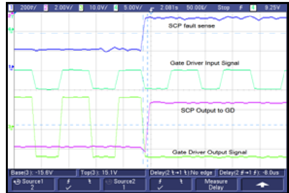
Figure 9. SCP tested with gate driver circuit and 10 nF load capacitor (Room temperature).
