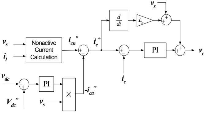
(b) Control diagram of the shunt compensation system
