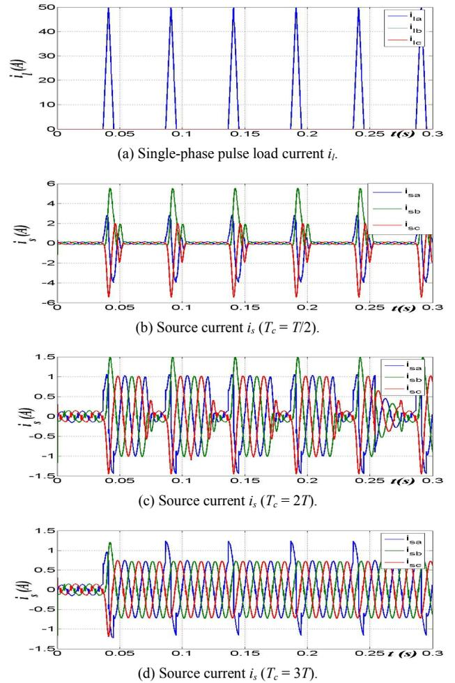
Fig. 5. Simulation of single-phase pulse load compensation.
