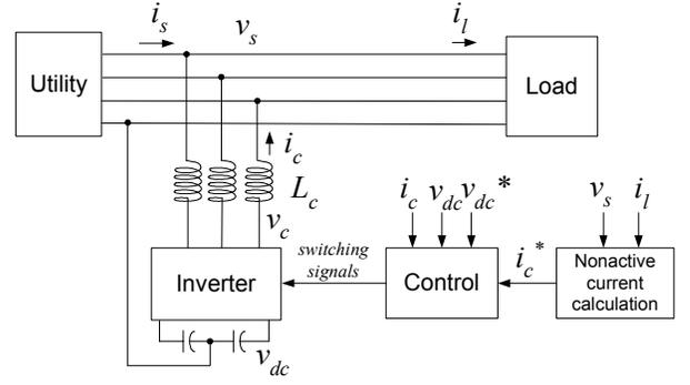
Fig. 1. System configuration of shunt nonactive power compensation.
