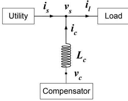
(a) Equivalent circuit of the compensation system
