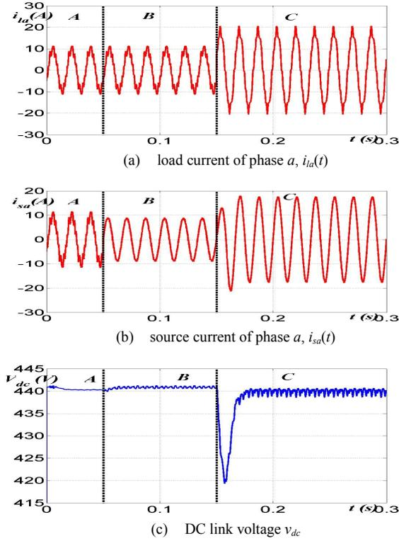
Fig. 3. Simulation of harmonic load compensation.
