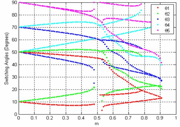
Fig. 2. Switching angle solutions to 5-angle unipolar switching scheme vs.  $m$ .
