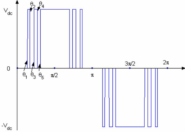
Fig. 1. Five-angle unipolar switching output.
