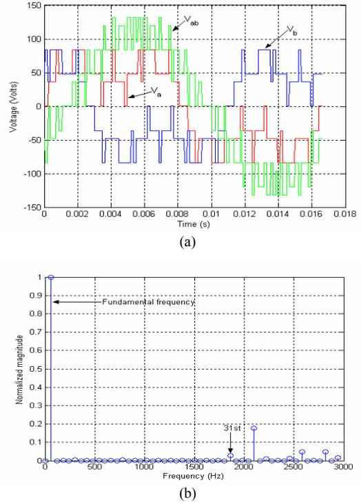
Fig. 11. Simulation of a 5-level case ( $k_1 = 0.75, k_2 = 1, V_{dc} = 48 \text{ V}, m = 1.080$ , THD = 19.19%) to eliminate harmonics up to 29th, (a) voltage waveform; (b) normalized FFT analysis of line-line voltage.
