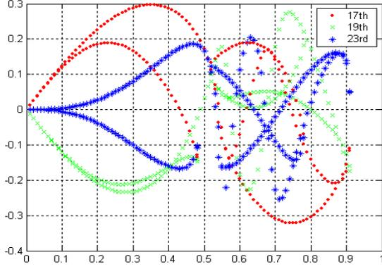
Fig. 4. Normalized 17th, 19th, and 23rd harmonic magnitudes vs.  $m$ .
