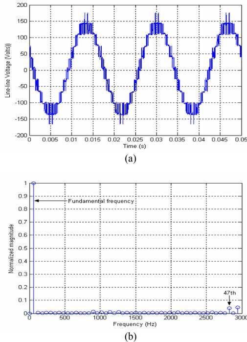
Fig. 13. Experimental voltages for 7-level case ( $k_1 = 0.9$ ,  $k_2 = 0.95$ ,  $k_3 = 1$ ,  $V_{dc} = 38$  V,  $m = 1.66$ , THD = 6.42%) to eliminate harmonics up to 43rd, (a) line-line voltage; (b) Normalized FFT analysis of line-line voltage
