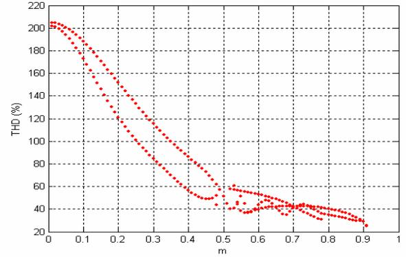
Fig. 3. THD vs.  $m$  for switching angles shown in Fig. 2.
