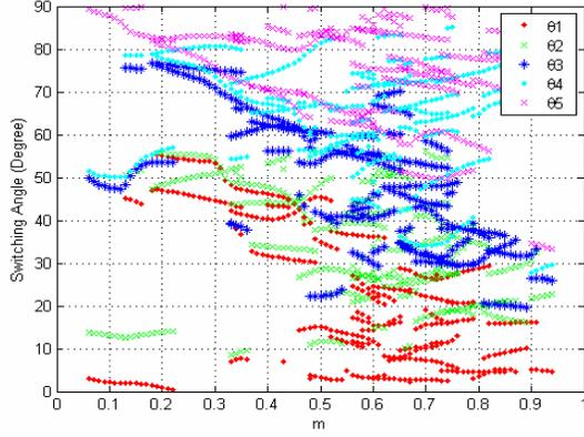
Fig. 8. Switching angles for 5-angle unipolar switching scheme to eliminate the 19th, 23rd, 29th and 31st harmonics vs.  $m$ .
