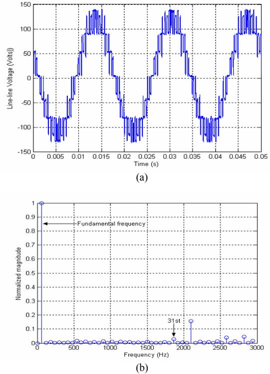
Fig. 12. Experiment of 5-level case ( $k_1 = 0.75, k_2 = 1, V_{dc} = 48 \text{ V}, m = 1.080$ , THD = 17.4%) to eliminate harmonics up to 29th, (a) line-line voltage; (b) normalized FFT analysis of line-line voltage.
