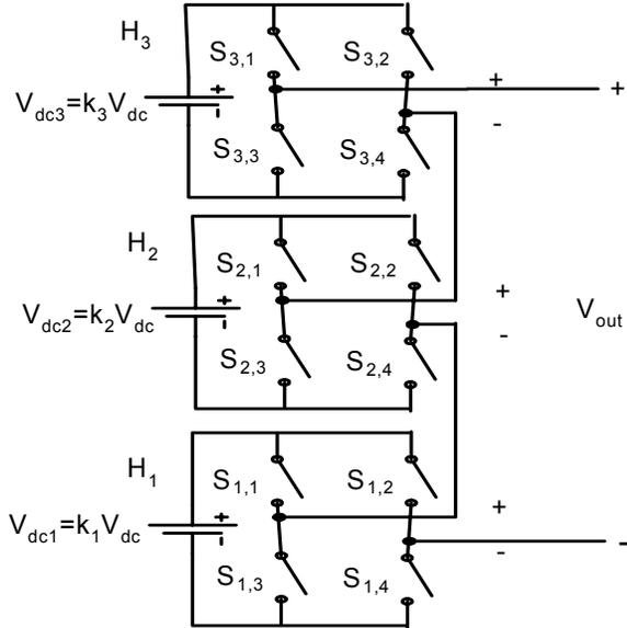
Fig. 9. Seven-level multilevel converter topology.
