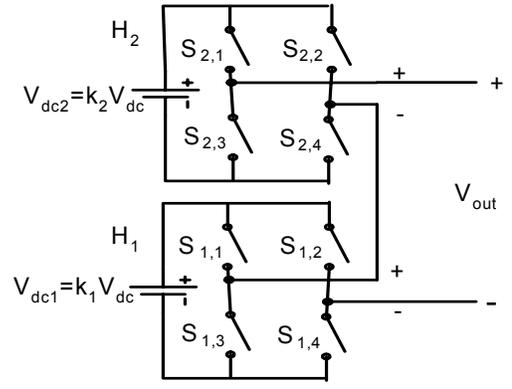
Fig. 5. Five-level multilevel converter topology.
