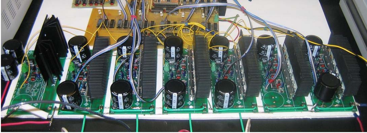
Fig. 6. The 6-level 5 kW version of the MMCCC with 6 modules. The sixth module (first one from right) is bypassed for normal operation.
