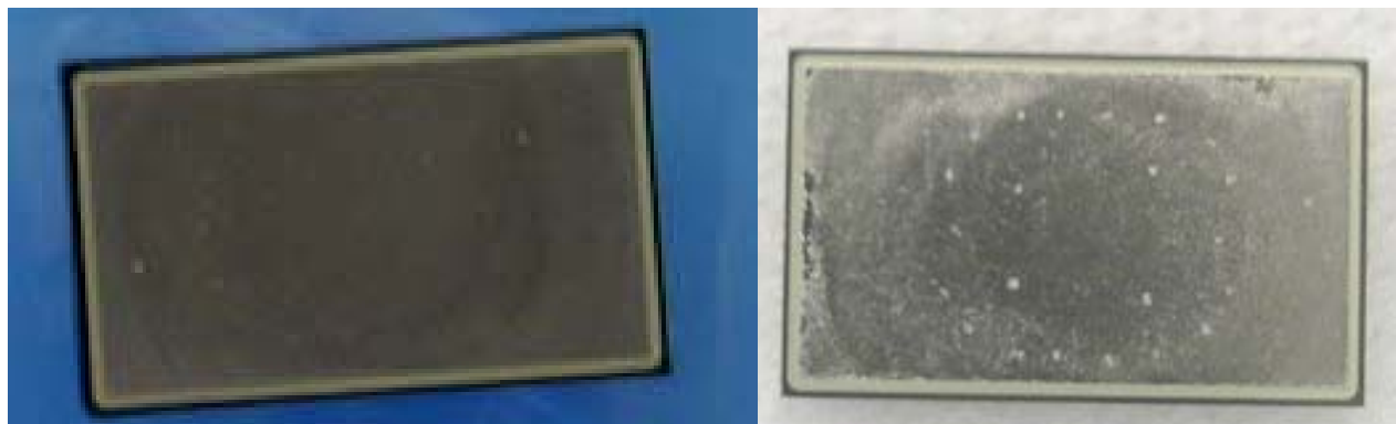
Figure 3: A 75 A, 1200V SiC diode (left) after zincating, (right) after EN plating.
