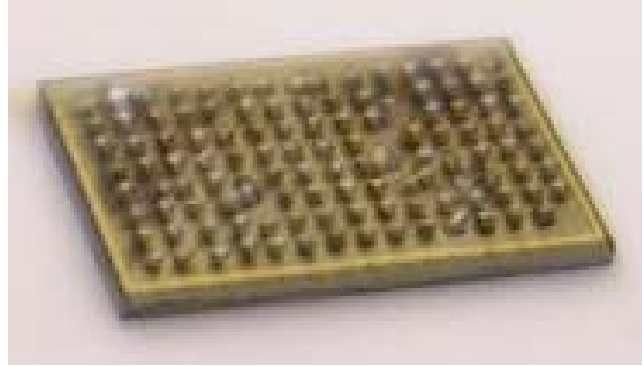
Figure 4: A bumped SiC diode prior to assembly into a prototype package.
