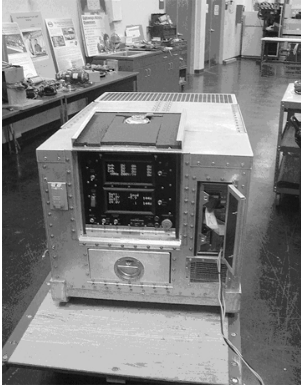
Figure 5. 1. Small 8-kW gen-set, control panel and display, computer access, cable connection access door, convenience plug. (P9220036)
