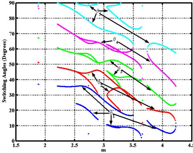
Fig. 3. Switching angles vs.  $m$  for a staircase waveform produced by a multilevel inverter with 5 H-bridges.
