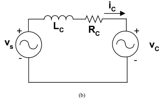
Fig. 5. (a) System configuration and (b) equivalent circuit of the SVC system.
