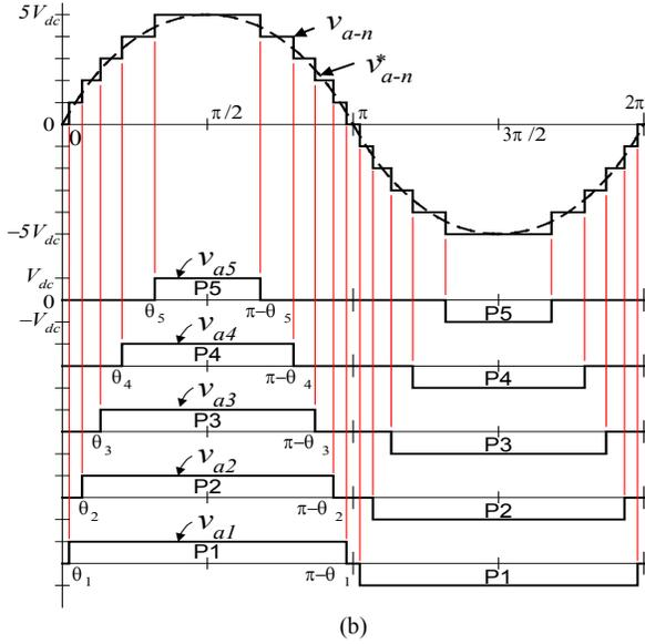
Fig. 1. (a) Multi-level cascaded H-bridges converter and (b) staircase output waveform.
