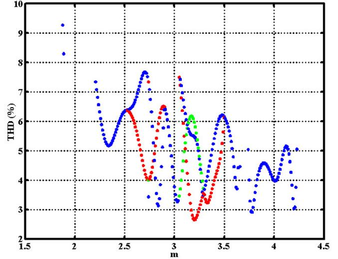
Fig. 4. The total harmonic distortion versus  $m$  for each solution set in Fig. 3.
