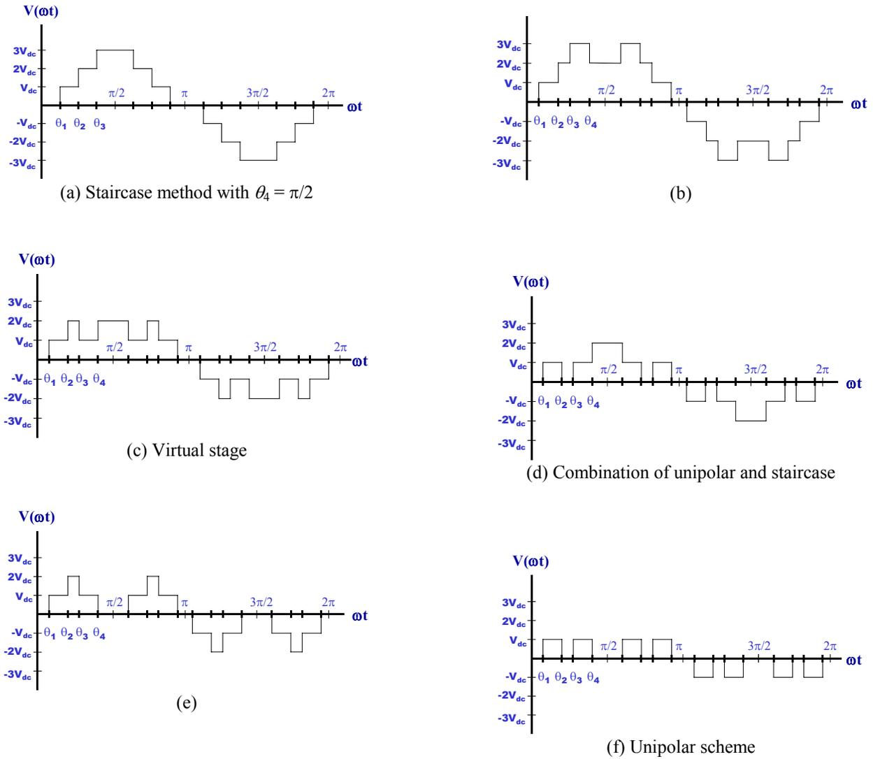
Fig. 2. Possible switching schemes for a multilevel inverter with  $s = 3$ .
