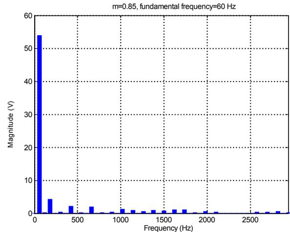
Fig. 12. FFT of the voltage waveform in Fig. 11.
