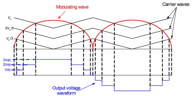
Fig. 5. Fundamental switching sine triangle wave comparison.
