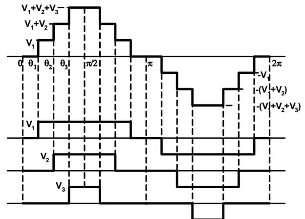
Fig. 4. n-level cascaded multilevel inverter waveform generation.
