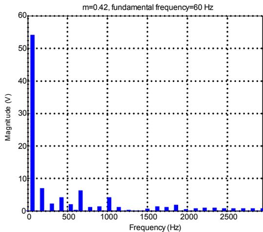
Fig. 10. FFT of the voltage waveform in Fig. 9.
