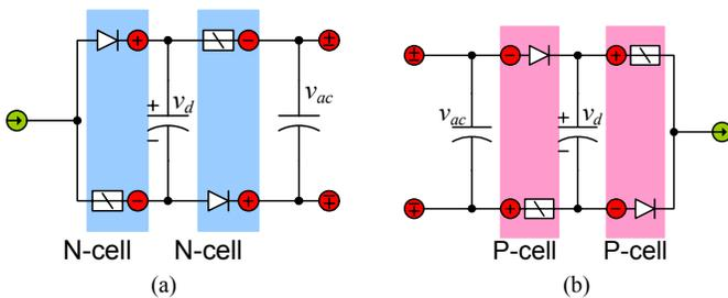
Fig. 9. Series connection of the N-cells and P-cells to form an ac voltage port.
