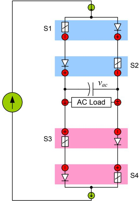
Fig. 8. Conventional current source inverter.
