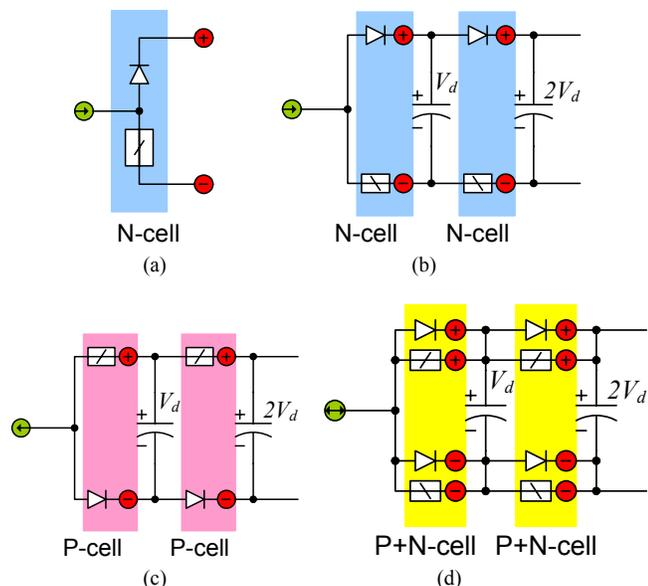
Fig. 7. A phase leg with bidirectional current flow by paralleling the P- and N-cells.
