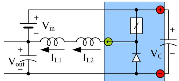
Fig. 3. Moving the two inductors of the P-cell Cuk converter (Fig. 2h) to the center rail and combining them into one.
