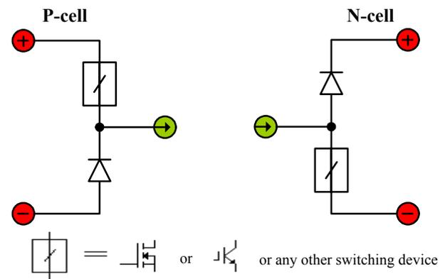
Fig. 1. Two basic switching cells: P-cell and N-cell. Terminal (+) connects to the positive lead of a voltage-source or capacitor, (−) connects to the negative lead of a voltage-source or capacitor, (→) connects to the positive lead of a current-source or inductor, and (←) connects to the negative lead of a current-source or inductor. The switching device  $\square$  can be a MOSFET, IGBT, or other controlled semiconductor switching device.
