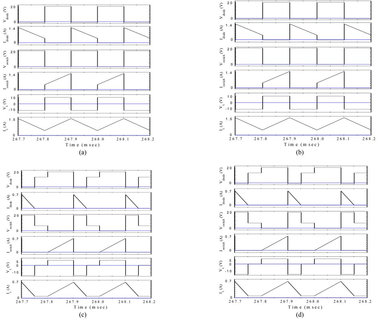
Fig. 5. Simulation results of (a) N-cell buck converter with continuous conduction, (b) P-cell buck converter with continuous conduction, (c) N-cell buck converter with discontinuous conduction, (d) P-cell buck converter with discontinuous conduction.
