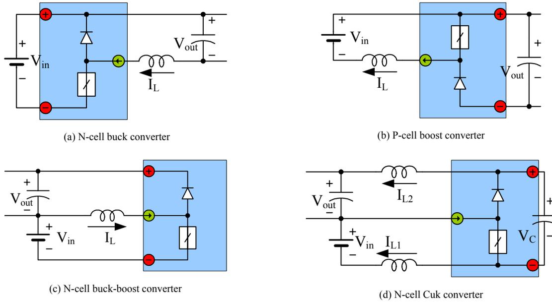
Fig. 4. The mirror circuits of the traditional dc-dc converters.
