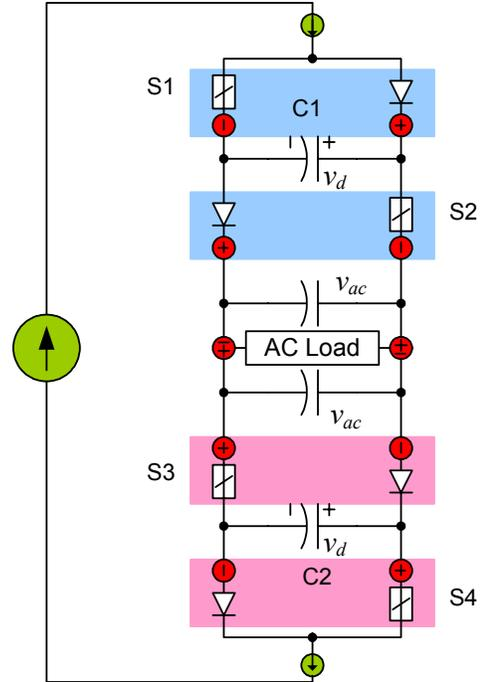
Fig. 10. Current source inverter constructed from series combination of P-cell and N-cell shown in Fig. 9.
