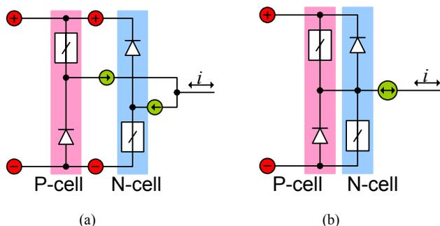
Fig. 6. A phase leg with bidirectional current flow by paralleling the P- and N-cells.
