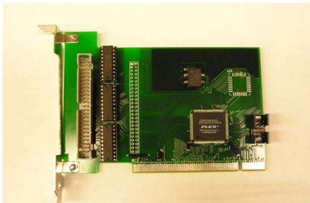
Fig. 7. FPGA controller for multilevel converter.
