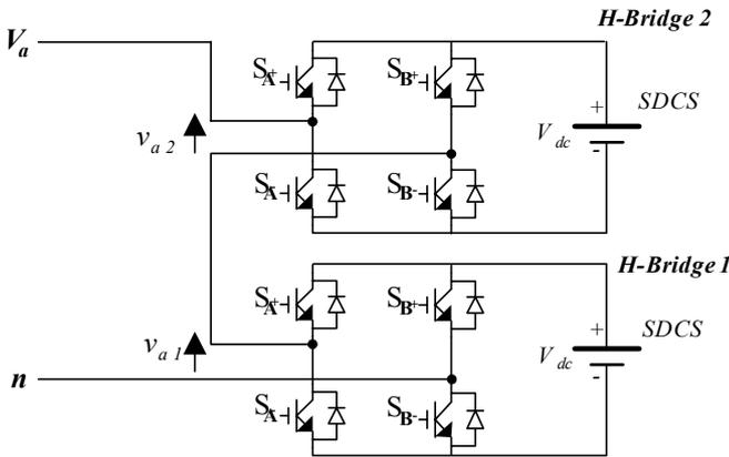
Fig. 1. Single-phase multilevel-inverter system
