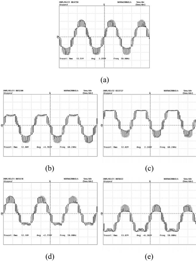
Fig. 8. Experiment of fault features at (a) normal, (b)  $S_{A+}$  fault, (c)  $S_{A-}$  fault, (d)  $S_{B+}$  fault, and (e)  $S_{B-}$  fault of H-bridge 2 with modulation index = 0.8 out of 1.0.
