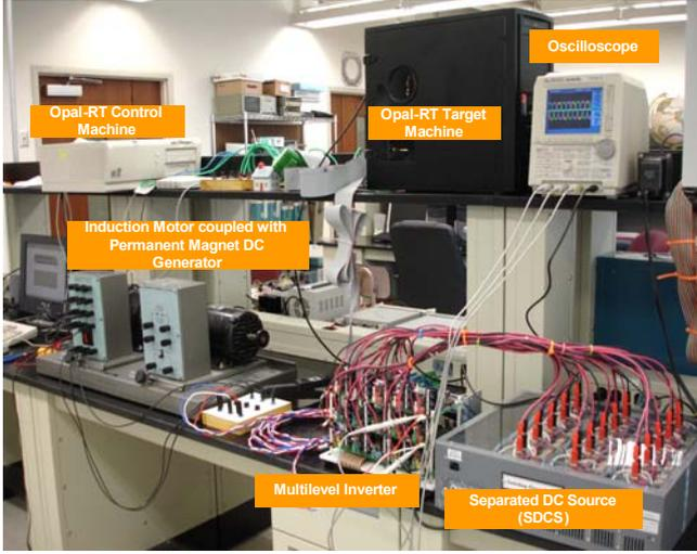
Fig. 7. Experiment setup.
