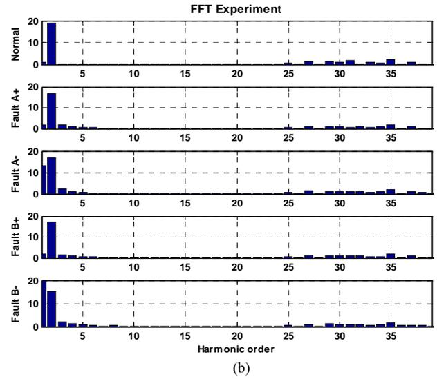
Fig. 4. (a) Simulation and (b) experimental results of fault features at  $S_{A+}$ ,  $S_{A-}$ ,  $S_{B+}$ , and  $S_{B-}$  of H-bridge 2 with modulation index = 0.8 out of 1.0.
