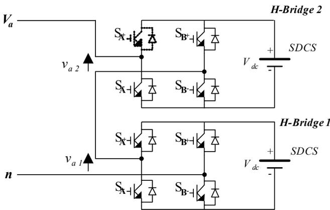
Fig. 2. H-Bridge 2, Switch  $S_{A+}$  open circuit fault at second level of single-phase multilevel-inverter.
