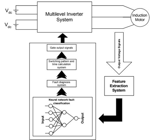
Fig. 3. Structure of fault diagnosis system.
