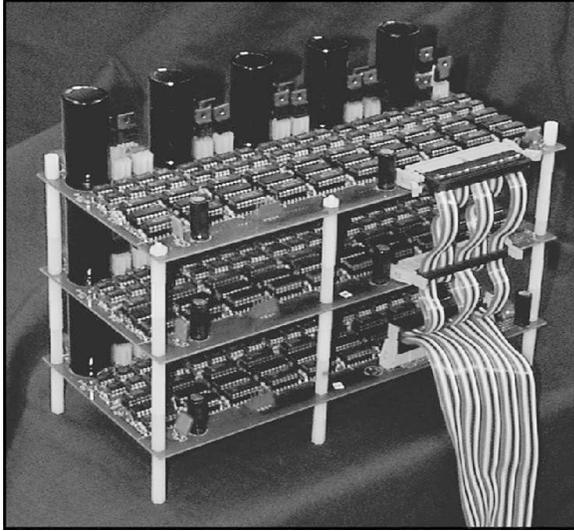
Fig. 7. Gate driver boards and MOSFETs for the multilevel inverter.
