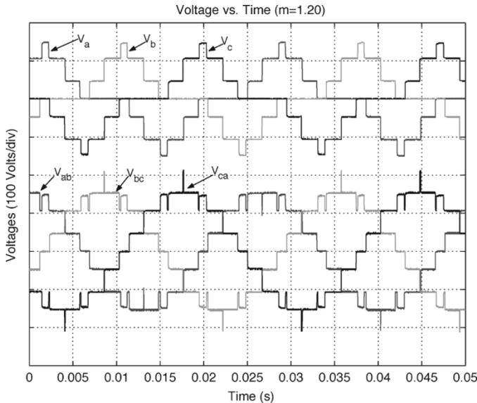
Fig. 8. Three-phase voltage waveforms for  $m_a = 0.4$  ( $m = 1.2$ ).
