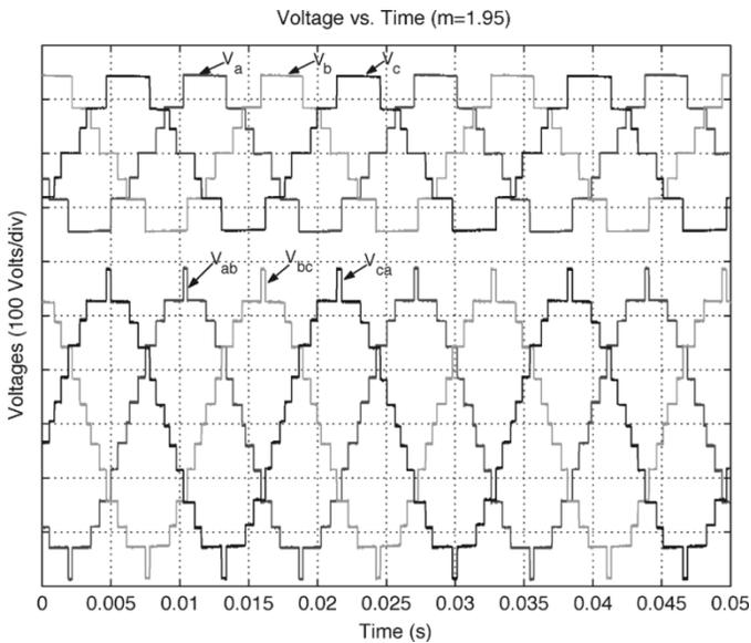
Fig. 12. Voltage waveforms for  $m_a = 0.65$  ( $m = 1.95$ ).
