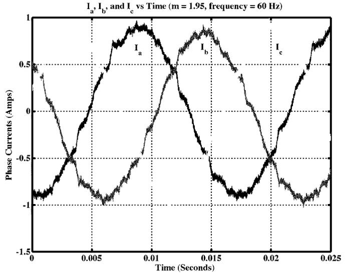
Fig. 14. Current waveforms for  $m_a = 0.65$  ( $m = 1.95$ ).
