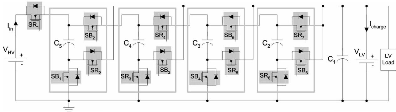
Fig. 3. Five-level MMCCC with four modular blocks.
