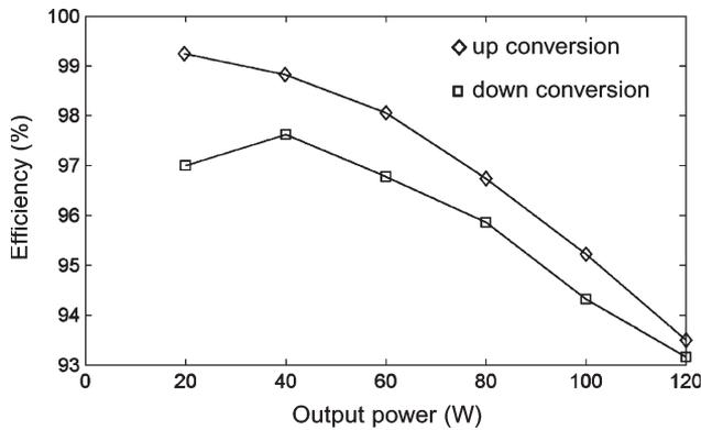
Fig. 13. Efficiency of the MMCCC at different power outputs.
