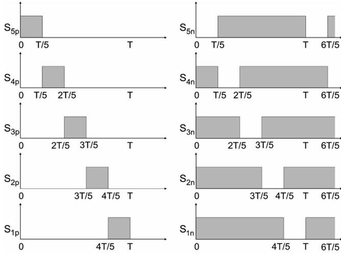
Fig. 2. Switching scheme of the FCMDC circuit.
