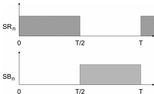
Fig. 6. Gating signal of the switches in the new circuit, i.e., there are only two switching states present in the circuit.
