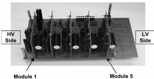
Fig. 14. 500-W six-level prototype.
