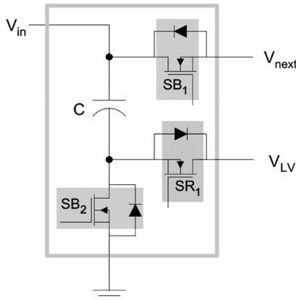
Fig. 4. Modular block of the MMCCC.
