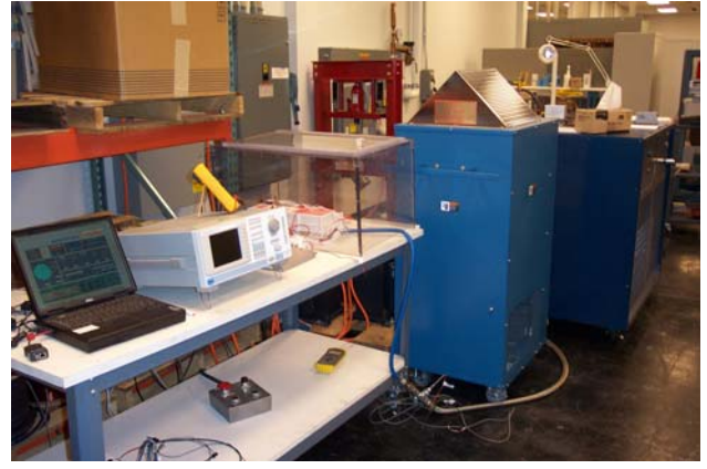
Fig. 4. Inductive load test set-up.
