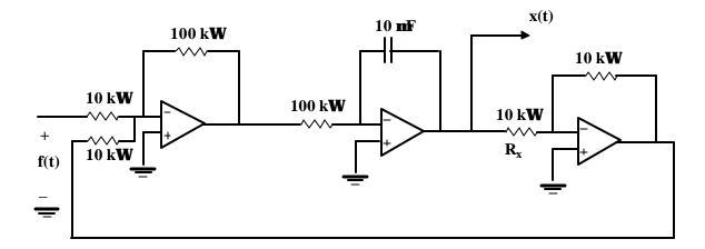
f(t) is the forcing function of a differential equation. x(t) is the dependent variable of this differential equation. The circuit above solves this differential equation.
