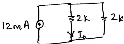
$$I_0 = 12\text{mA} \left( \frac{2k}{2k+2k} \right) \\ = 6\text{mA}$$
