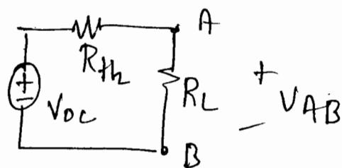
$$V_{AB} = V_{DC} \left[ \frac{R_L}{R_L + R_{Th}} \right]$$
