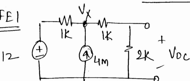
$$\frac{V_X - 12}{1\text{k}} + \frac{V_X}{3\text{k}} - 4\text{mA} = 0$$
