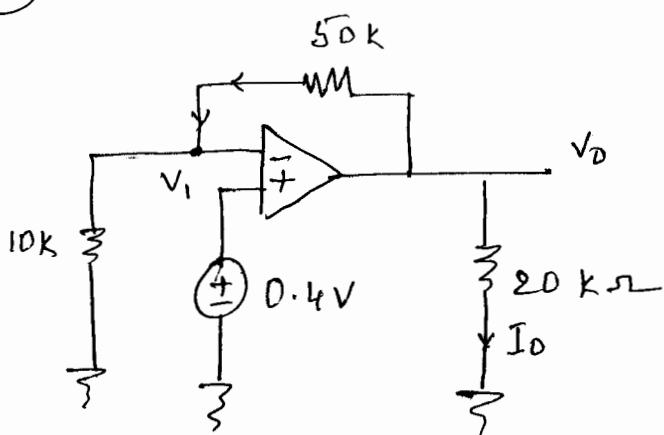
$$\frac{V_0 - V_1}{50k} = \frac{V_1}{10k} \quad V_1 = 0.4 \text{ V}$$
