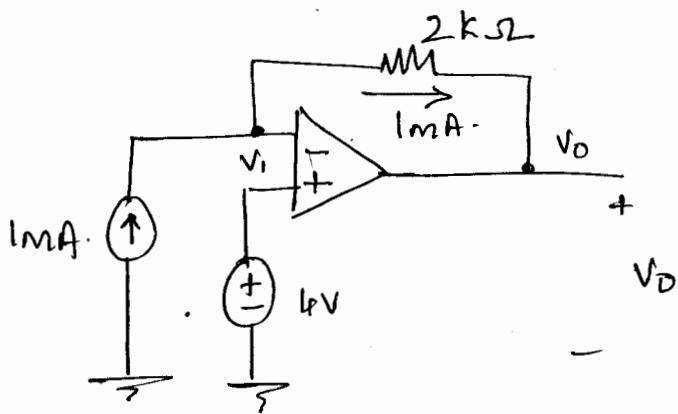
$$\text{Voltage at } V_1 = 4 \text{ V}$$
