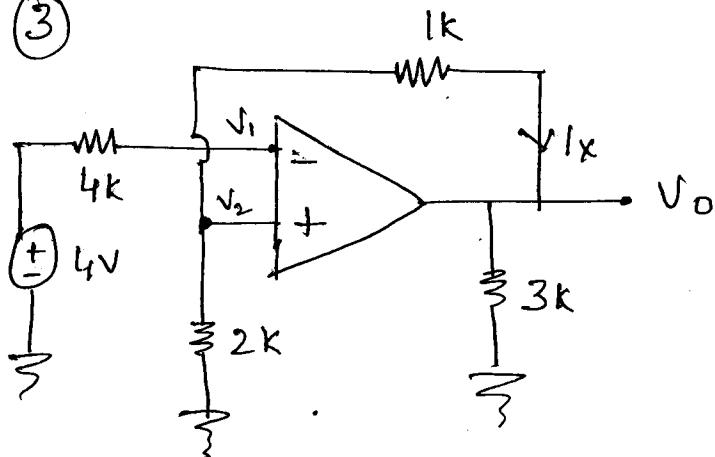
$V_1 = 4V$  as no current goes into the inverting terminal
