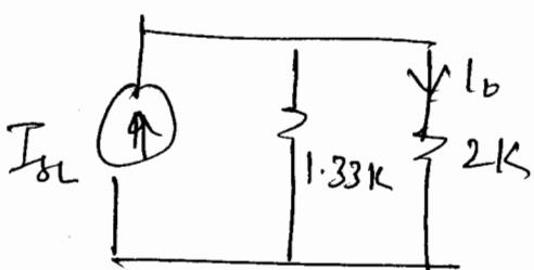
$$I_o = I_{sc} \left[ \frac{R_{out}}{R_{out} + 2k} \right]$$
