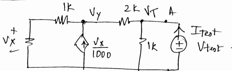
Apply a test source  $V_{test}$
