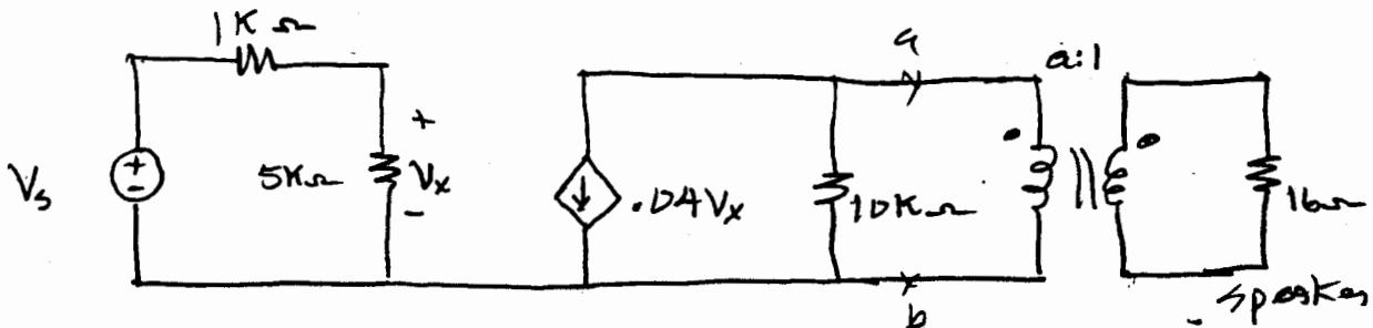
Select "a" so that the output impedance of the transistor amplifier matches the reflected resistance of the speaker.
