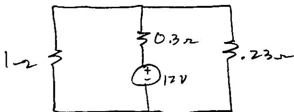
$$\hat{V}_{R_1} = \frac{12 \times \left( \frac{.23 \times 1}{1 + .23} \right)}{.3 + \left( \frac{.23 \times 1}{1 + .23} \right)} = 4.59 \text{ V}$$
