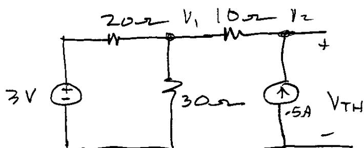
$$\frac{V_1 - 3}{20} + \frac{V_1}{30} + \frac{V_1 - V_2}{10} = 0 \quad \dots$$
