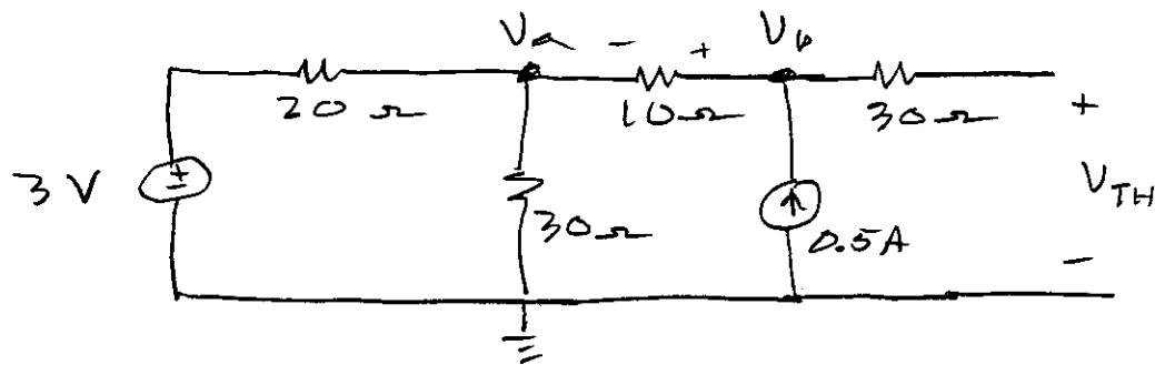
No current flows in the  $30\ \Omega$  resistor since that portion of the circuit is open. Thus, no voltage drop. Thus  $V_{TH} = V_b$
