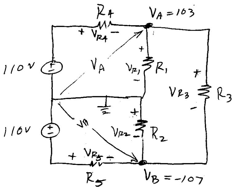
$$\boxed{V_{R_1} = V_A = 103 \text{ V}}$$
