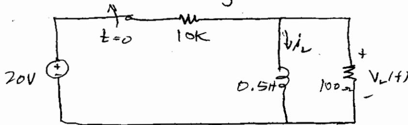
(a) Develop the DE that allows you to solve for  $V_L(t)$ .
