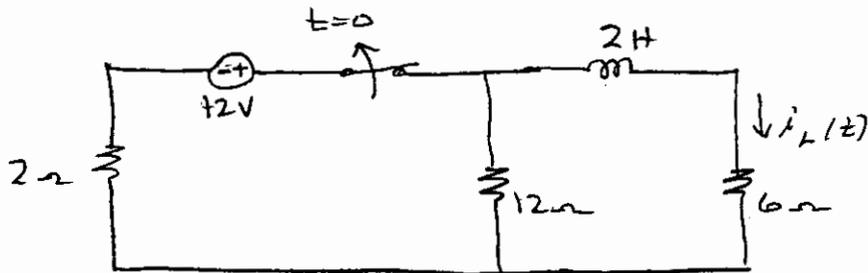
With the switch closed for a long time, the inductor is a short circuit. We can find  $i_L(0^-)$  from the following:
